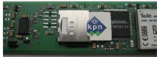
^ SIM card installed on PCB, 2 GB Micro SD memory card is positioned under SIM card holder.
